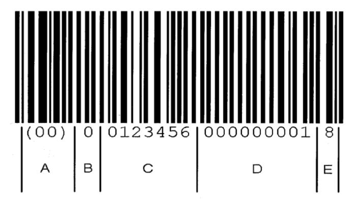
The UCC-128 20-digit barcode is a sequential, serialized bar code that represents a case from a manufacturer or vendor. It consists of five parts:
