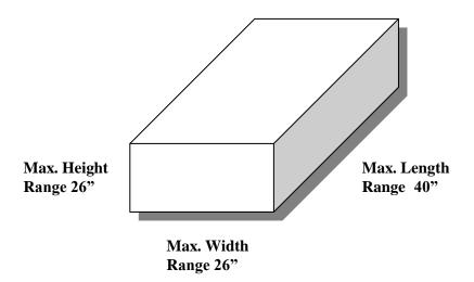
**Conveyable Cases** - This diagram shows the maximum dimensions for a conveyable case. This is the largest case that can be transported by our conveyors. "Arrow" placement or "This Side Up" directions on box does not effect UCC-128 label placement.
